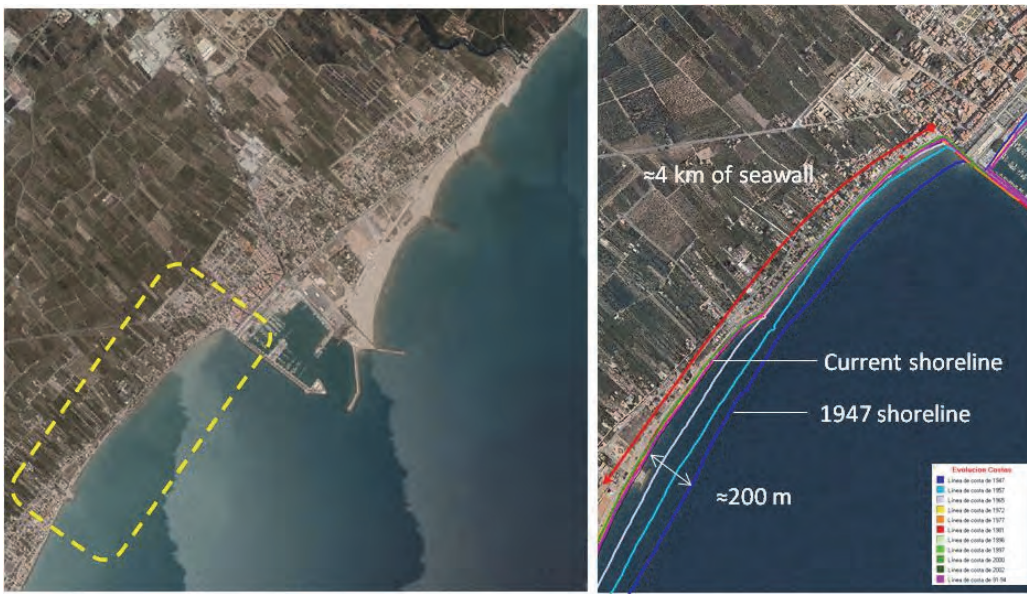
Fig.2 Port and southern coast of Burriana: seashore evolution. Source: Coastal Information System (Valencian Regional Government).
