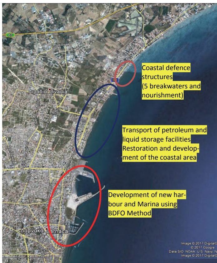
Fig.4 Main areas and elements of intervention
