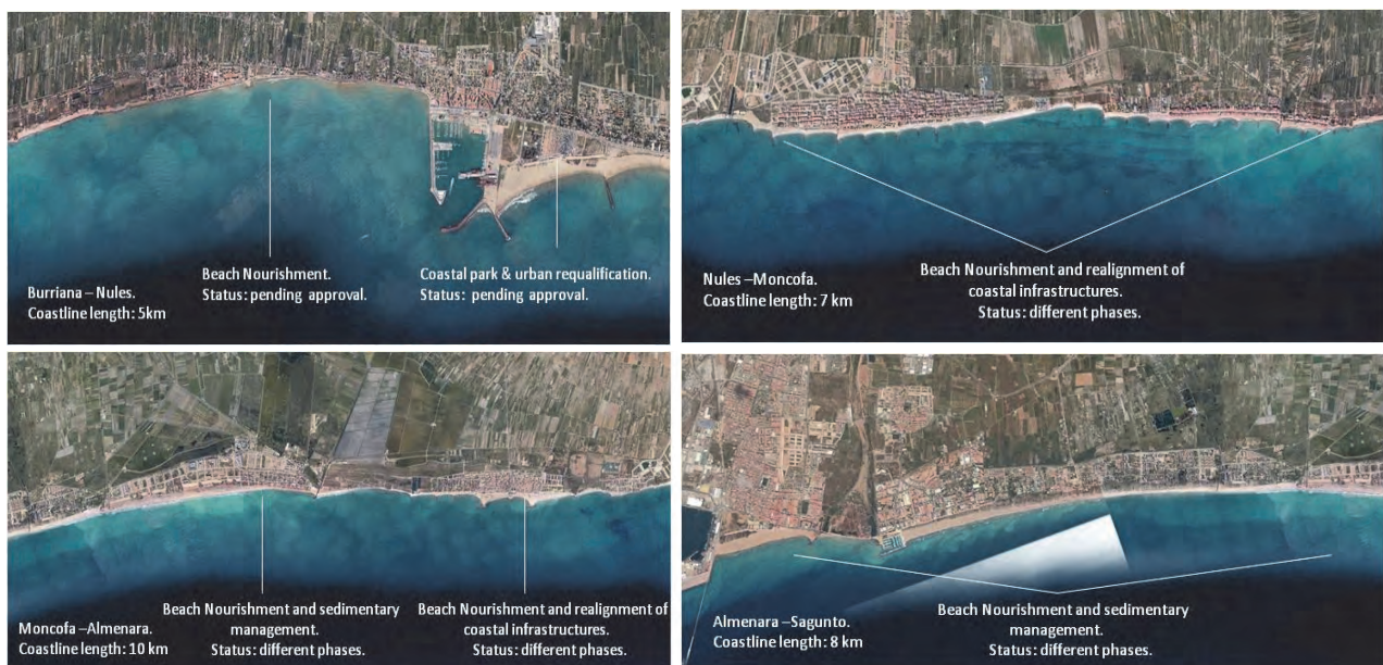
Fig. 3 Project coastal stretches from north (Port of Burriana) to south (Port of Sagunto). Source: Google Earth.
